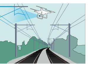
In airborne field trials, the system has detected small, static obstacles above ground clutter, including powerlines, metal poles, people, and cars at ranges out to hundreds of metres. Doppler processing has also been used to identify moving objects including small drones and birds.
